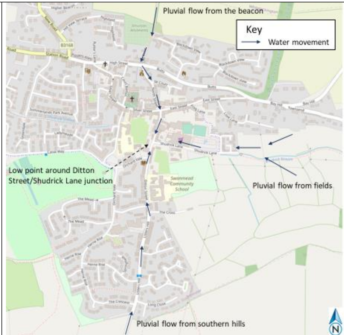
Figure 31: Pluvial flows around east Ilminster
